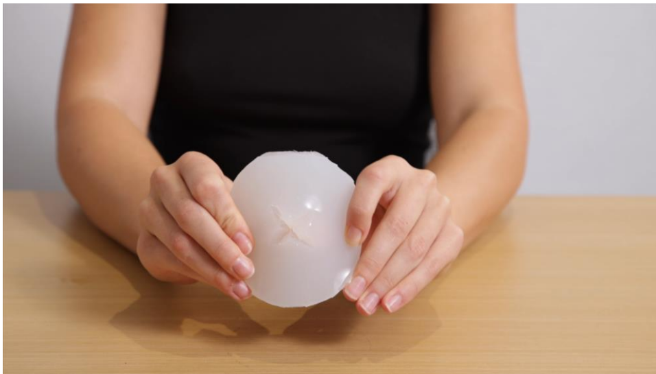
Silicone pad with an X cut in the middle
