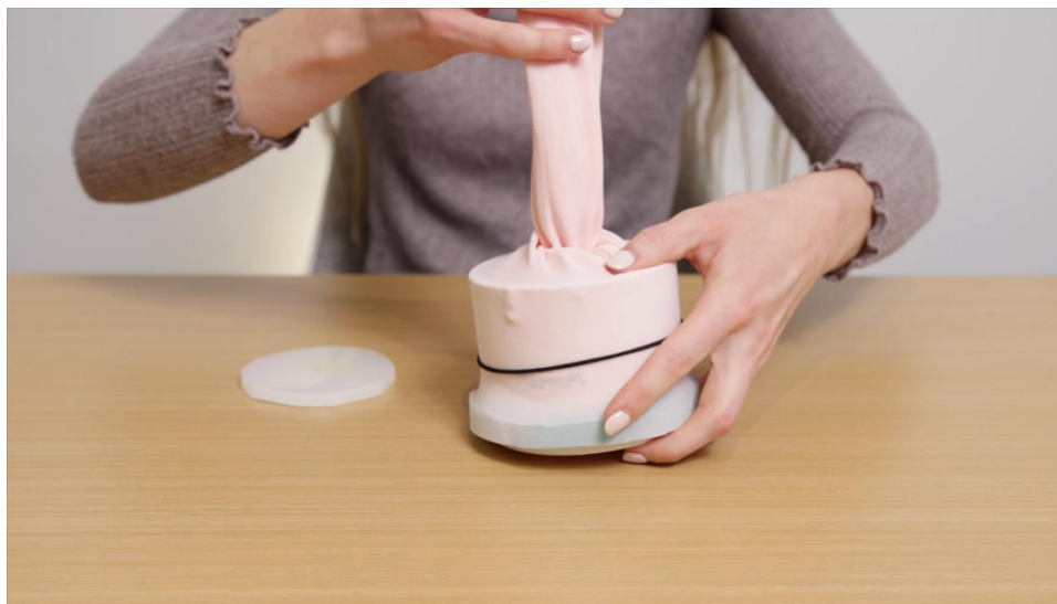
Image 5 – Outer layer of tights wrapped around PVC vagina and secured with a hair tie
